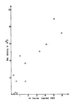
Increase of <sup>15</sup>O activity in NO with increasing amounts of injected NO. For 5 ml injected NO, the specific activity after separation corresponds to approximately 1.5  $\mu$ c/m mole and the product contains about 30 % of the activity originally present in 0<sup>15</sup>O.
